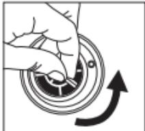
To replace the filter, remove the bottle cap, rotate the filter in an anti-clockwise direction and remove it by pulling it upwards.
