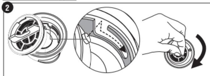
Insert the filter in its housing
